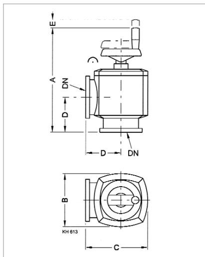
These universal valves are ideal especially for smaller systems, where remote control is not essential. They may be also installed in larger systems, where backing pumps or condensate separators or similar units are to be cut off at longer intervals for maintenance purposes by maintenance personnel.
