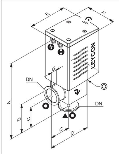
Dimensional drawing for the bellows-sealed right-angle valves
