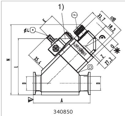
Dimensional drawing for the straight-through valves with fitted pilot valve (EP) without pilot valve (P)
