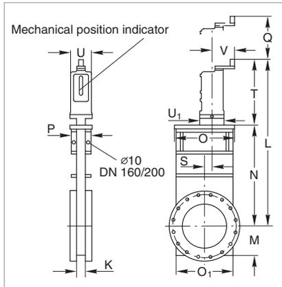
Dimensional drawing for the UHV gate valves
