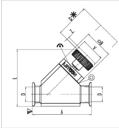
Dimensional drawing for the manually operated, bellows-sealed straight-through valves
