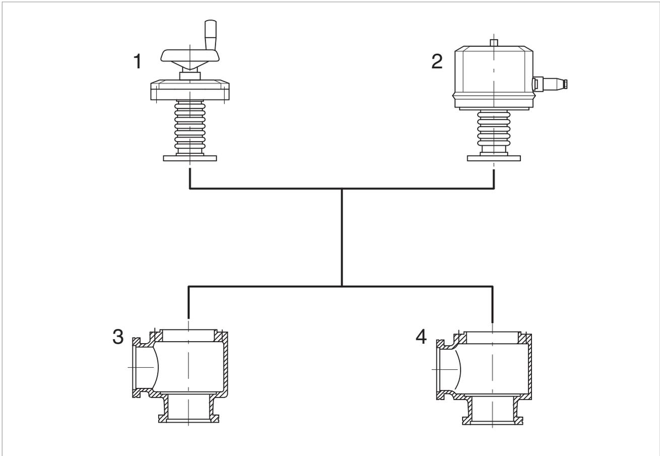
Oerlikon Leybold Vacuum valves with ISO-K flanges are available with any of two drives and either of two bodies.
